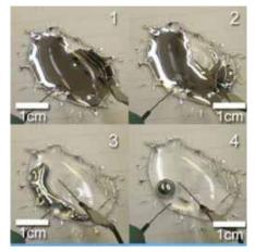
Snapshots of liquid metal transformation from a film to a sphere
