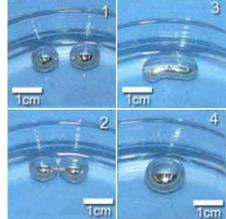
Snapshots of two separate droplets combining into a fused sphere from stage 1 to 4
