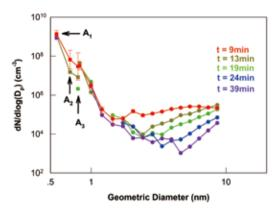
Time-dependent particle size distributions formed by gas-phase nucleation in a chamber
